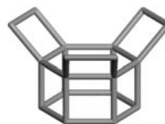
Figure 11. A possible secondary structural building unit that may dictate columnar growth in zeolite L.
